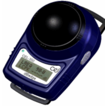
CEL-350 dBadge micro noise dosimeter
